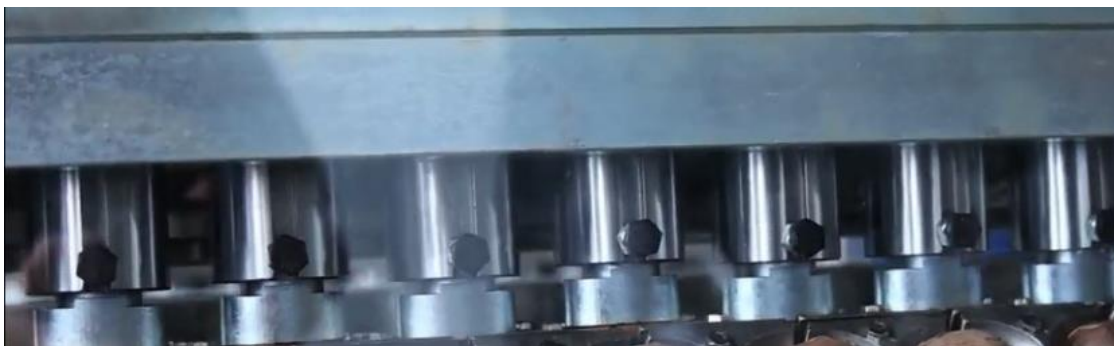
Cracking head and indexed nut positioning pockets
